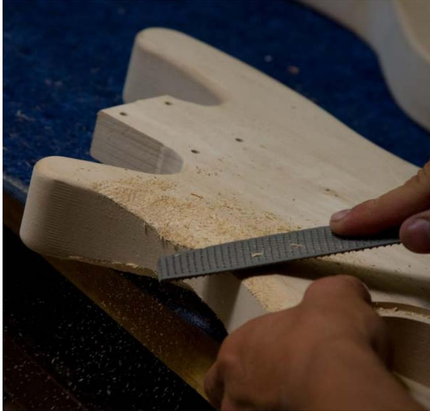
**Figure 6 – Shaping a Body with a Rasp**
