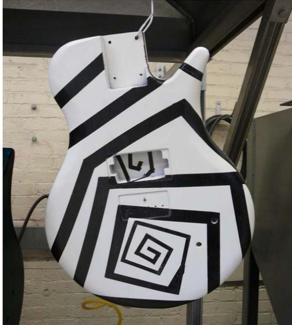
**Figure 8** – A Two Color Instrument before the Clear Coat
