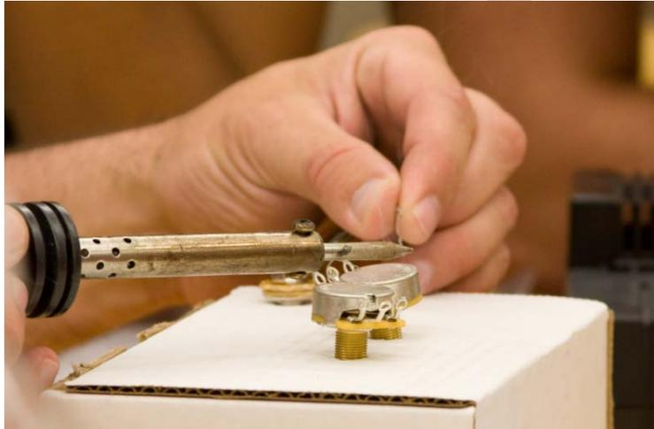
**Figure 36** – Making a Wiring Harness
