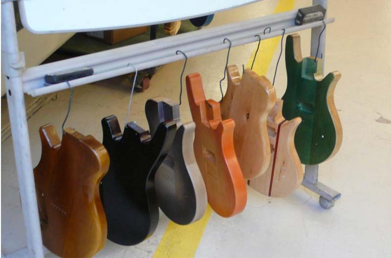
**Figure 7** – Guitar Bodies Drying After Finishing
