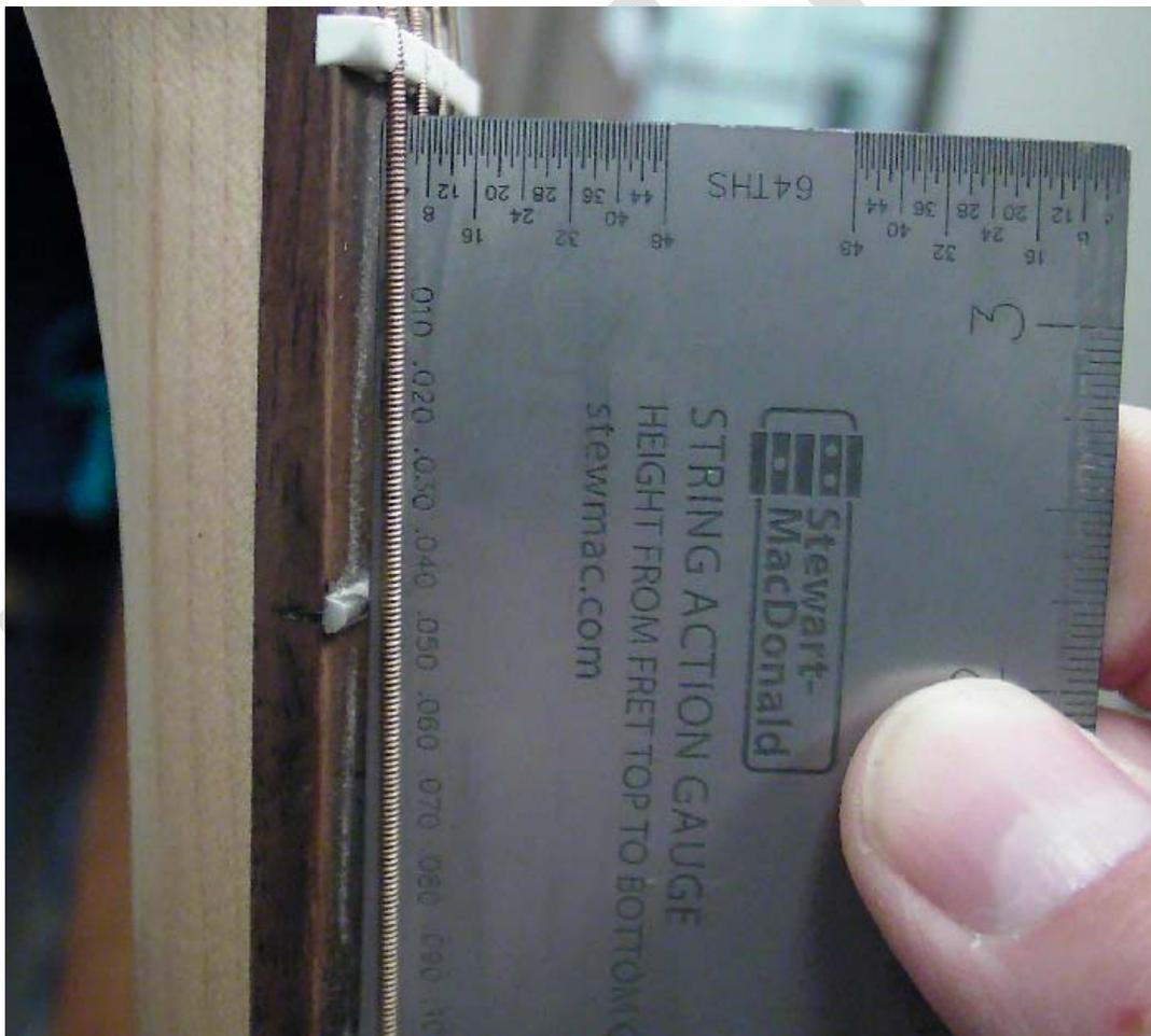
**Figure 60** – Using String Action Gauge
