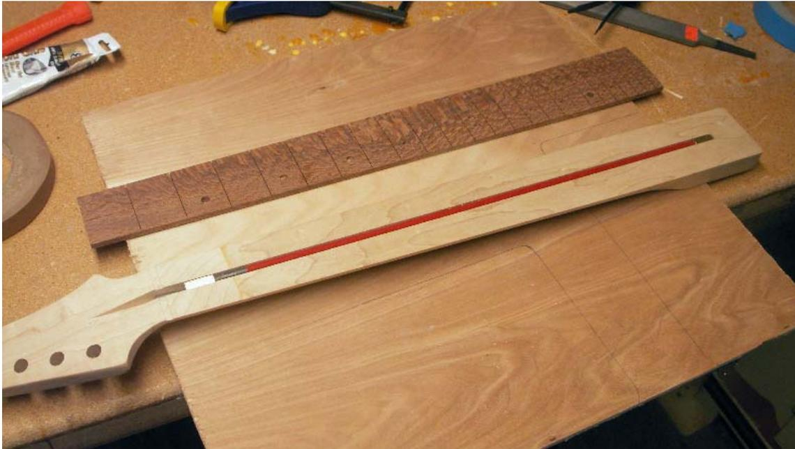
**Figure 12** – Neck with Truss Rod and Fretboard
