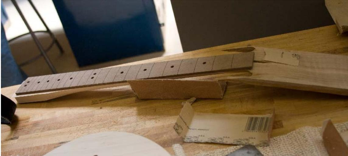
**Figure 15** – Fretboard with Dot Holes Drilled
