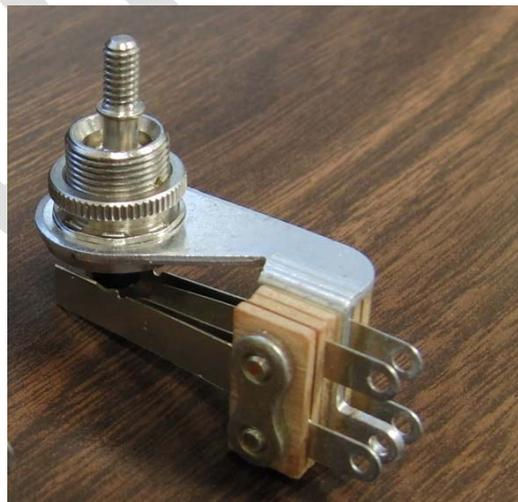
**Figure 37** – A Typical Three Way Switch
