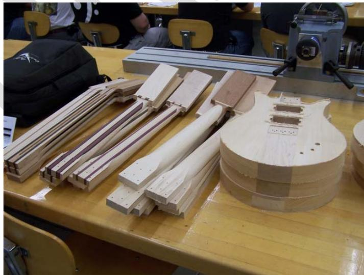
**Figure 1** – Rough Milled Necks and Bodies
