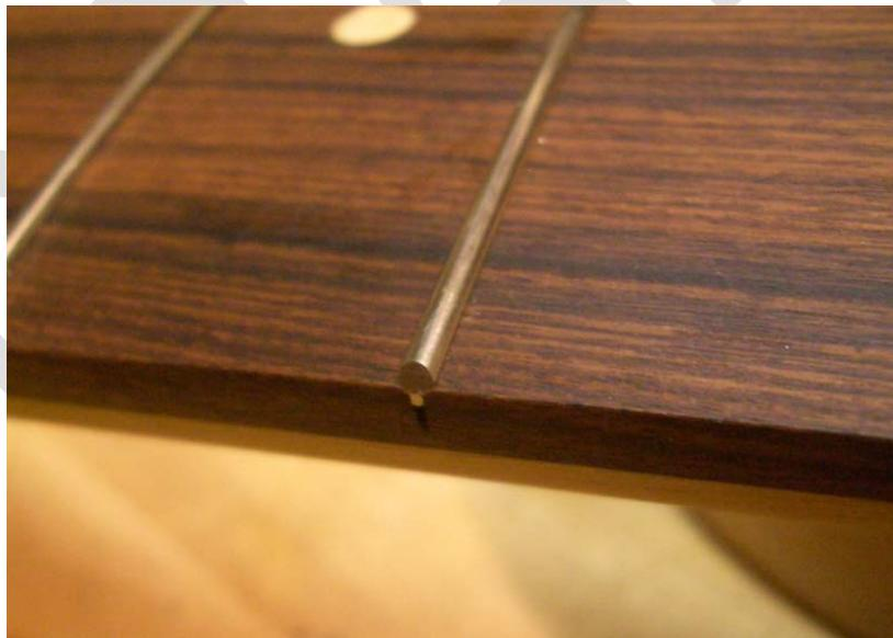
**Figure 35** – A Correctly Dressed Fret End
