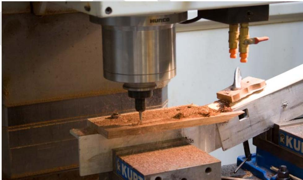
**Figure 11** – Headstock Being Milled
