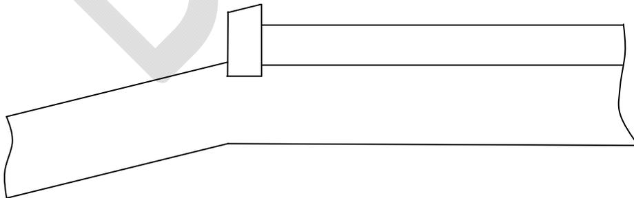
**Figure 48** – Taper the String Nut towards the Headstock
