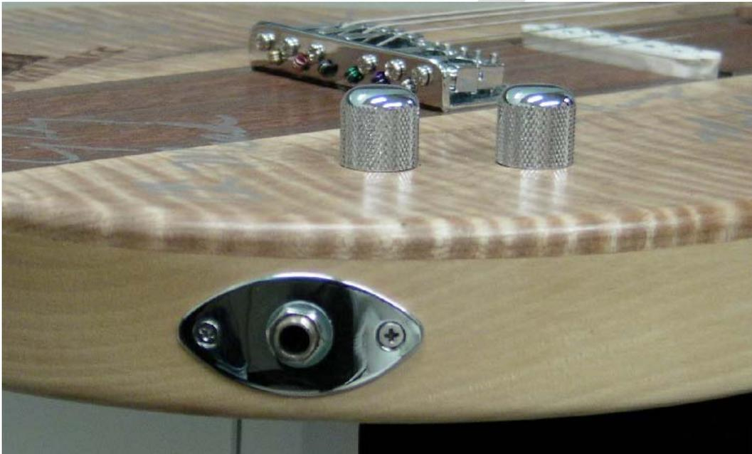
**Figure 40** – Jack Plate Secured to the Body
