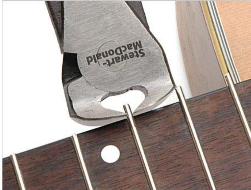
**Figure 31** – Trimming the Fret Ends Flush (image courtesy of Stewart MacDonal, [www.stewmac.com](http://www.stewmac.com))
