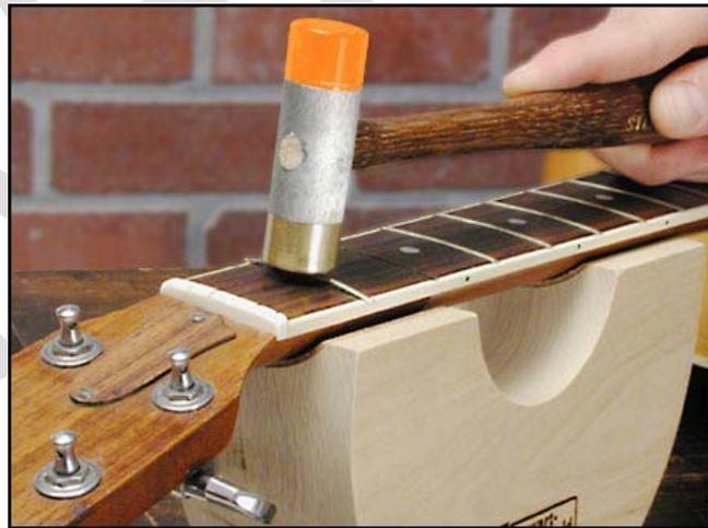
**Figure 28** – Seating the Center of a Fret with a Fretting Hammer (image courtesy of Stewart MacDonald, [www.stewmac.com](http://www.stewmac.com))
