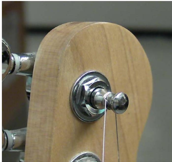
**Figure 58** – String Wound onto Tuner Post
