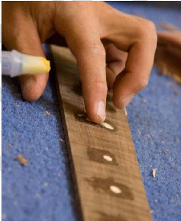
**Figure 16** – Gluing Wood Dots into the Fretboard
