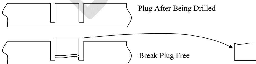
**Figure 14** – Cutting Wood Plugs from a Board
