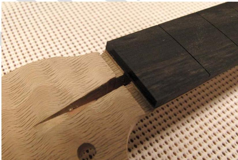
**Figure 19** – Fretboard Correctly Aligned on Neck
