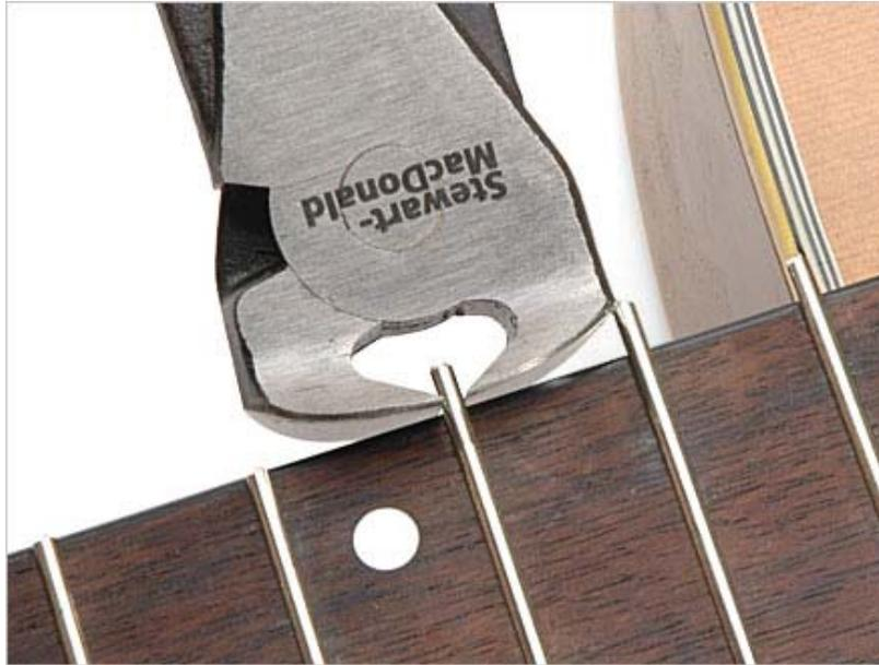
**Figure 31** – Trimming the Fret Ends Flush (image courtesy of Stewart MacDonald, [www.stewmac.com](http://www.stewmac.com))
