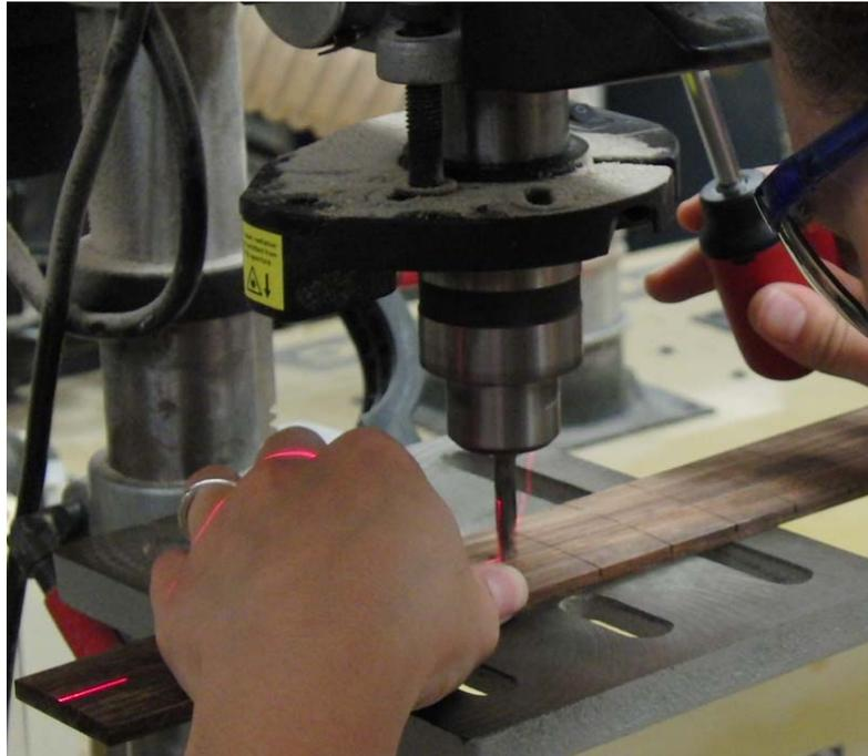
**Figure 13** – Drilling Holes for Fretboard Dots
