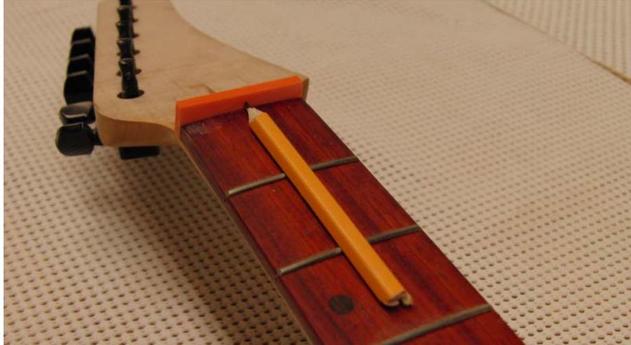
**Figure 46** – Marking the Neck Radius on the Nut
