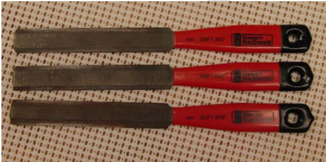
**Figure 51** – Nut Slotting Files
