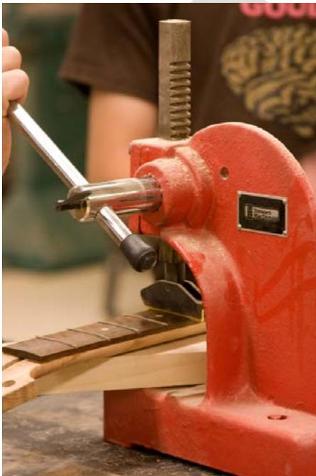
**Figure 27** – Arbor Press for Installing Frets (image courtesy Stewart MacDonald, [www.stewmac.com](http://www.stewmac.com))
