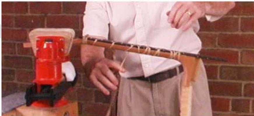
**Figure 21** – Heavy Rubber Bands Being used to Clamp a Fretboard to a Neck (picture courtesy of Stewart MacDonald, [www.stewmac.com](http://www.stewmac.com))
