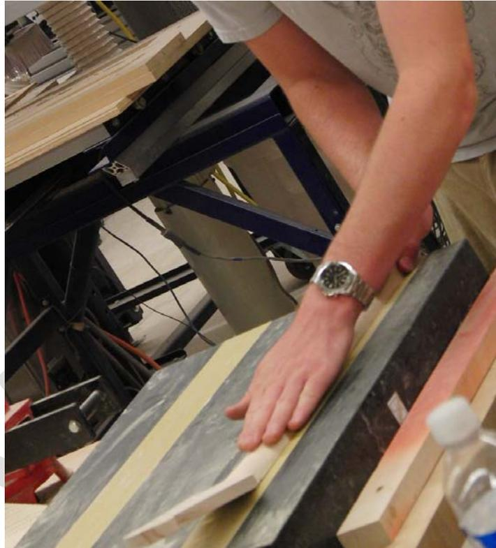
**Figure 17** – Flattening Neck Before Gluing on Fretboard
