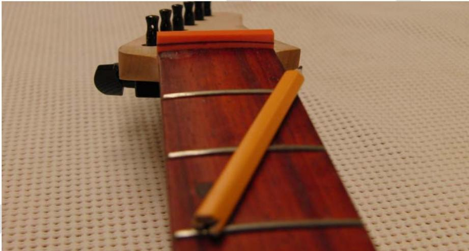
**Figure 47** – String Nut with the Radius Marked Correctly
