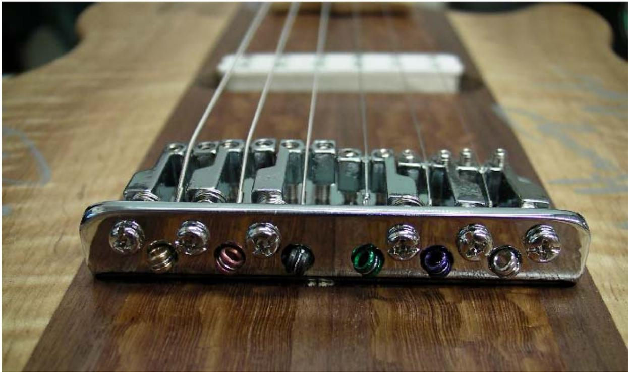
**Figure 62** – Intonation Adjustment Screws
